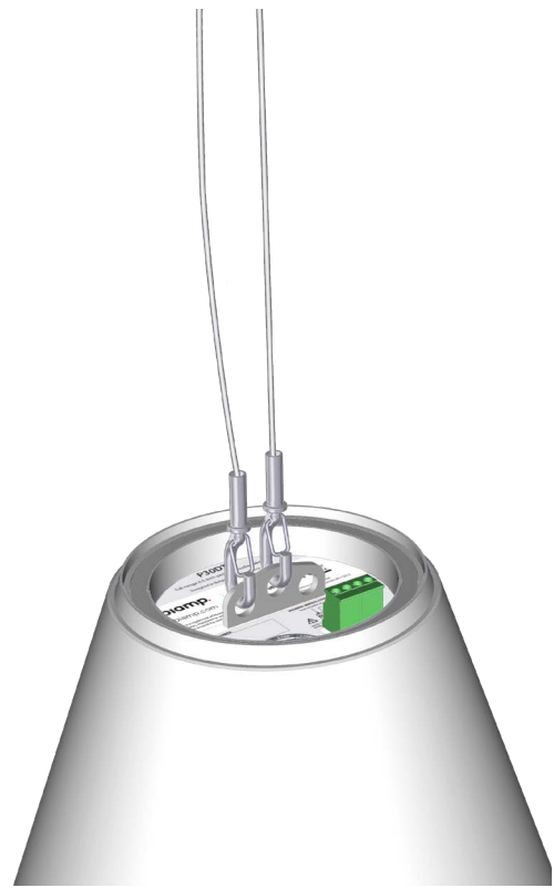
Figure 3. Attach secondary (safety) cable snaphook in a different bracket hole
