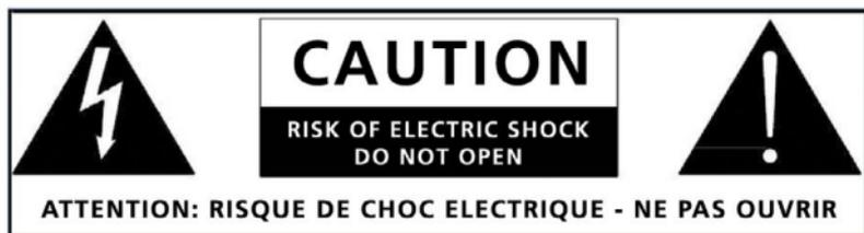
24. This lightning flash with arrowhead symbol within an equilateral triangle is intended to alert the user to the presence of non-insulated “dangerous voltage” within the product’s enclosure that may be of sufficient magnitude to constitute a risk of electric shock.
