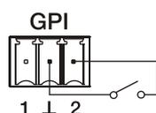
Figure 1: Connection example of GPI 2
