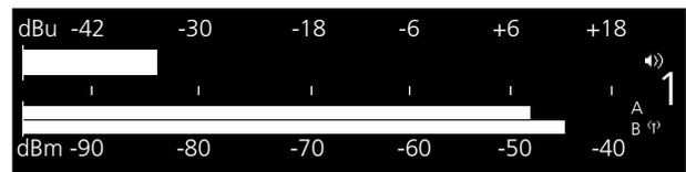
Combined audio and RF level display – transmitter turned on
