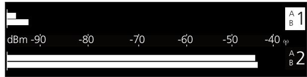
RF level display – interference on channel 1
