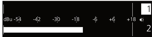
Audio level display – transmitter muted on channel 1
